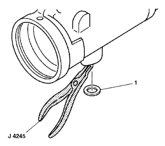
**Fig. 80: Installing Retaining Ring Using J 4245 (700 Gear)** Courtesy of GENERAL MOTORS CORP.
