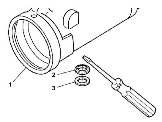
Fig. 76: Prying Backup Washer & Double Lip Seal From Steering Gear Housing Courtesy of GENERAL MOTORS CORP.
