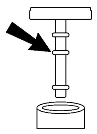
**Fig. 4: Removing Pump Reservoir Cap** Courtesy of GENERAL MOTORS CORP.
