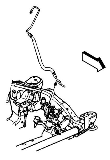
**Fig. 34: Power Steering Gear Inlet Hose & Power Steering Gear Courtesy of GENERAL MOTORS CORP.**
