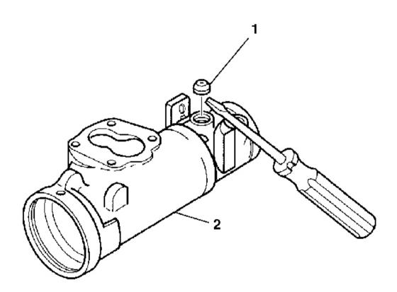
**Fig. 82: Removing Check Valve From Steering Gear Housing** Courtesy of GENERAL MOTORS CORP.
