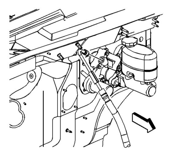
**Fig. 37: Brake Booster Inlet Hose & Brake Booster Courtesy of GENERAL MOTORS CORP.**
