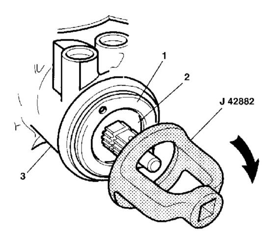
**Fig. 46: Turning Adjuster Nut Assembly Clockwise Using J 42882** Courtesy of GENERAL MOTORS CORP.
