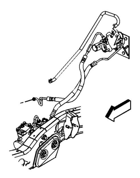
**Fig. 33: Power Steering Gear Inlet Hose & Brake Booster** Courtesy of GENERAL MOTORS CORP.
