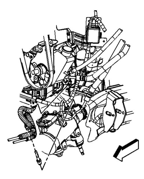
**Fig. 28: Identifying Hoses** Courtesy of GENERAL MOTORS CORP.
