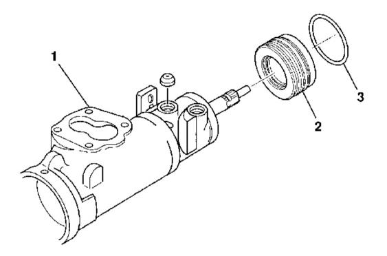
**Fig. 87: O-Ring Seal & Thrust Support Assembly Courtesy of GENERAL MOTORS CORP.**
