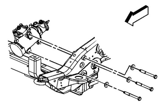
**Fig. 43: Power Steering Gear** Courtesy of GENERAL MOTORS CORP.
