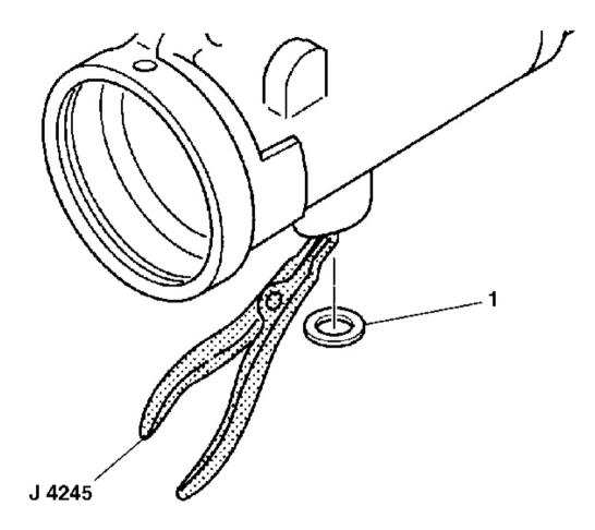
**Fig. 75: Installing Retaining Ring Using J 4245 (700 Gear)** Courtesy of GENERAL MOTORS CORP.
