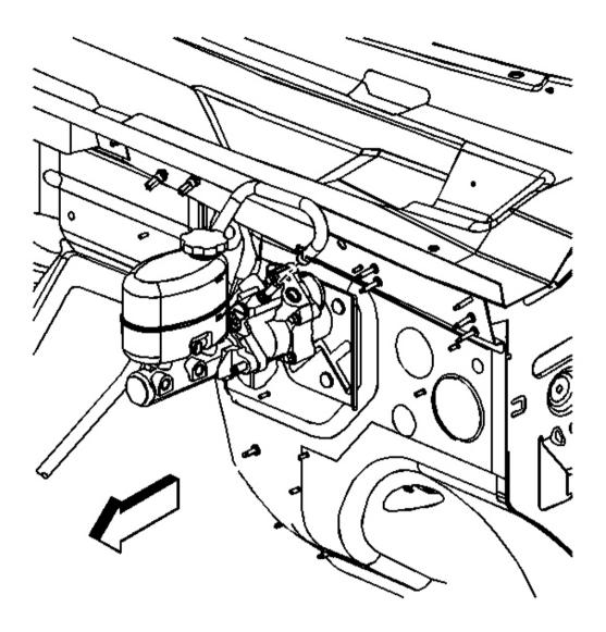
**Fig. 41: Brake Booster Outlet Hose & Brake Booster Courtesy of GENERAL MOTORS CORP.**
