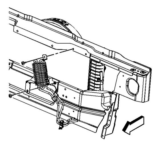
**<u>Fig. 30: Power Steering Cooler</u> Courtesy of GENERAL MOTORS CORP.**
