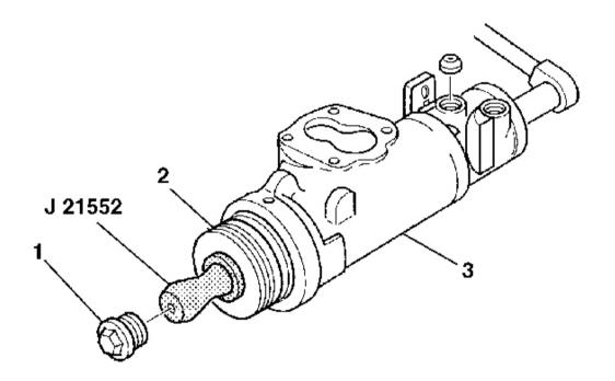
**Fig. 66: Turning Stub Shaft Counterclockwise Until Rack Piston Begins To Come Out Of Steering Gear Housing Courtesy of GENERAL MOTORS CORP.**
