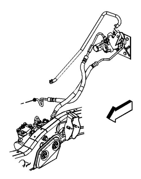
**Fig. 31: Power Steering Gear Inlet Hose & Brake Booster** Courtesy of GENERAL MOTORS CORP.
