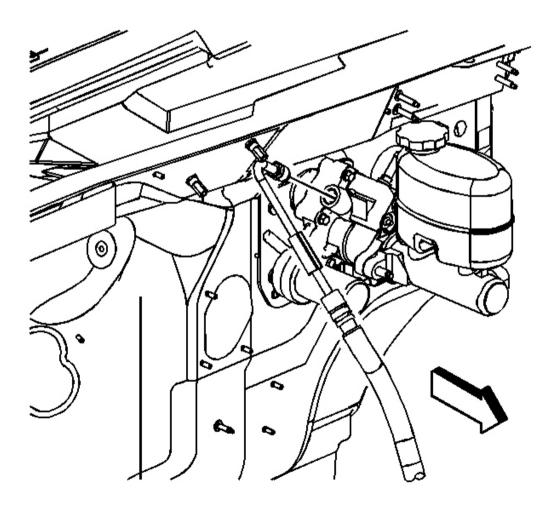
**Fig. 35: Brake Booster Inlet Hose & Brake Booster Courtesy of GENERAL MOTORS CORP.**
